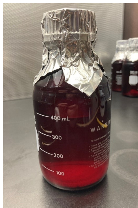
Oryzalin solution with precipitate visible at the bottom of the bottle. Photo courtesy of Bob Hamilton.
